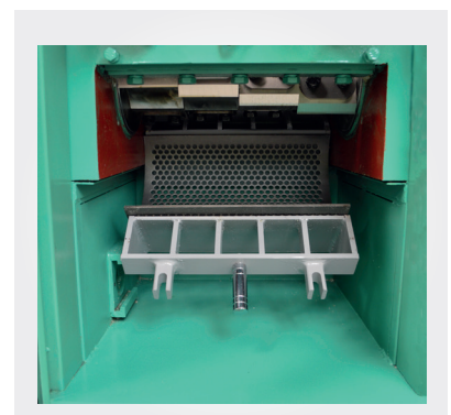
Easy access for maintenance and cleaning.
