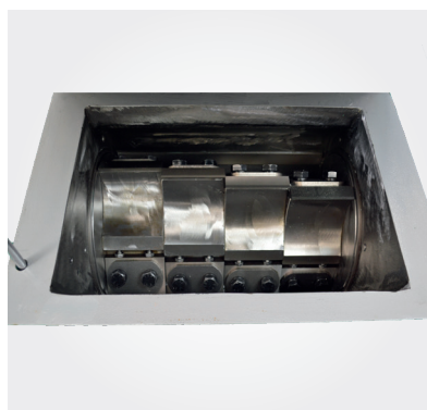
Staggered blade configuration for maximum efficiency.
